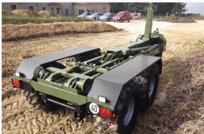
Bras reconditionné, Freinage AIR 40km/h, RC 560/60 R22.5, Pompe engrenages 118l/min, attelage Calotte
