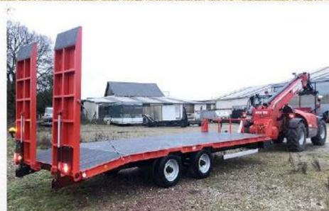
Surface utile : 7m00 x 2m54, Tandem susp. lame de ressorts, RC 235/75 R17.5, Pompe à main
