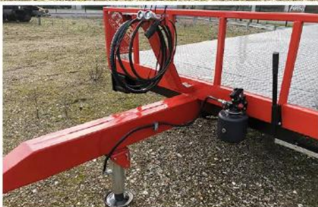
Surface utile : 7m00 x 2m54, Tandem susp. lame de ressorts, RC 235/75 R17.5, Pompe à main Sarl BCM - D910 La Normandie - 37110 VILLEDOMER - 02.47.550.100 - www.remorques-bcm.com
