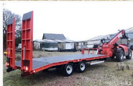
Surface utile : 7m00 x 2m54, Tandem susp. lame de ressorts, RC 235/75 R17.5, Pompe à main Sarl BCM - D910 La Normandie - 37110 VILLEDOMER - 02.47.550.100 - www.remorques-bcm.com
