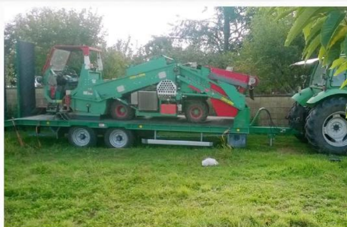
Surface utile : 7m00 x 2m54, Essieux fixes, RC 215/75 R17.5, Rampes larges (0m90)
