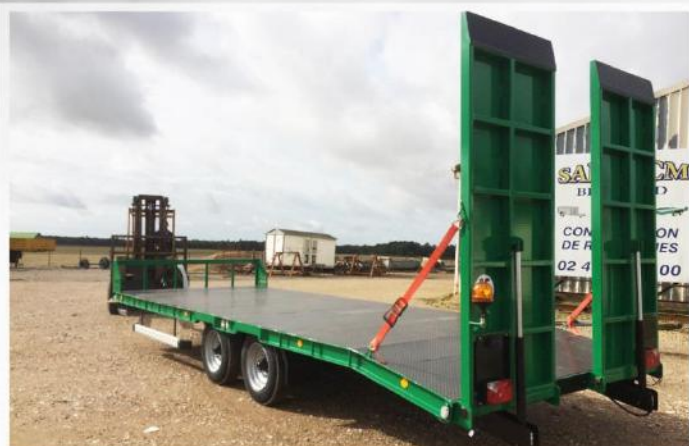
Surface utile : 7m00 x 2m54, Essieux fixes, RC 215/75 R17.5, Rampes larges (0m90)
